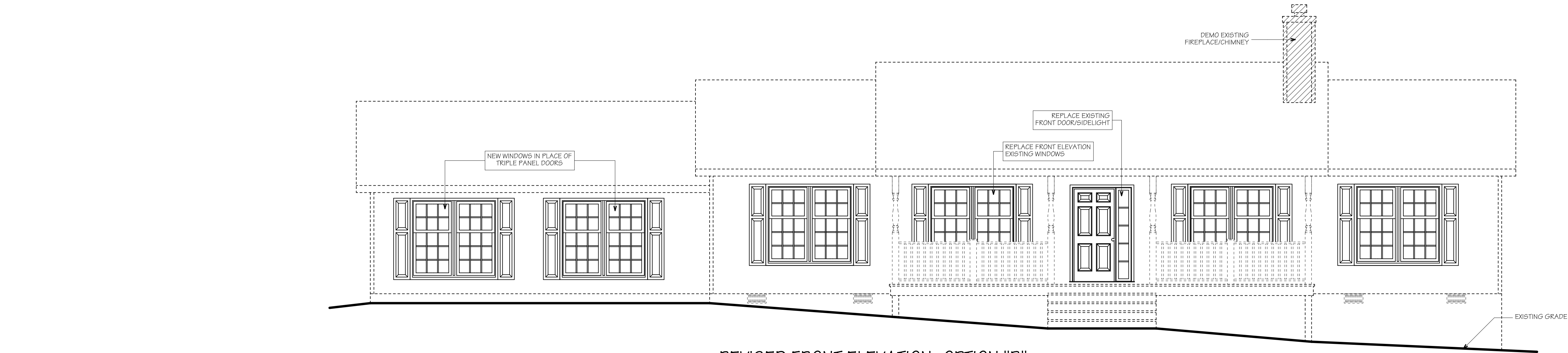
2D REVISED FRONT ELEVATION- OPTION "B" ALL COLOR AND FINISH SELECTIONS FOR MATERIALS SHOWN ARE BY OWNER SCALE: 1/4" = 1'-0"
